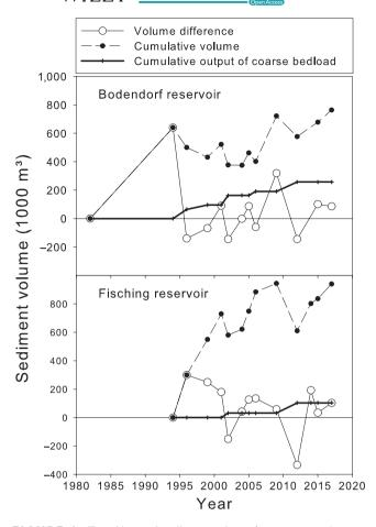
**FIGURE 4** Trend in total sediment volume (zero = start of operation), volume difference between echo sounding surveys, and output of coarse bed load for Bodendorf and Fisching reservoirs
